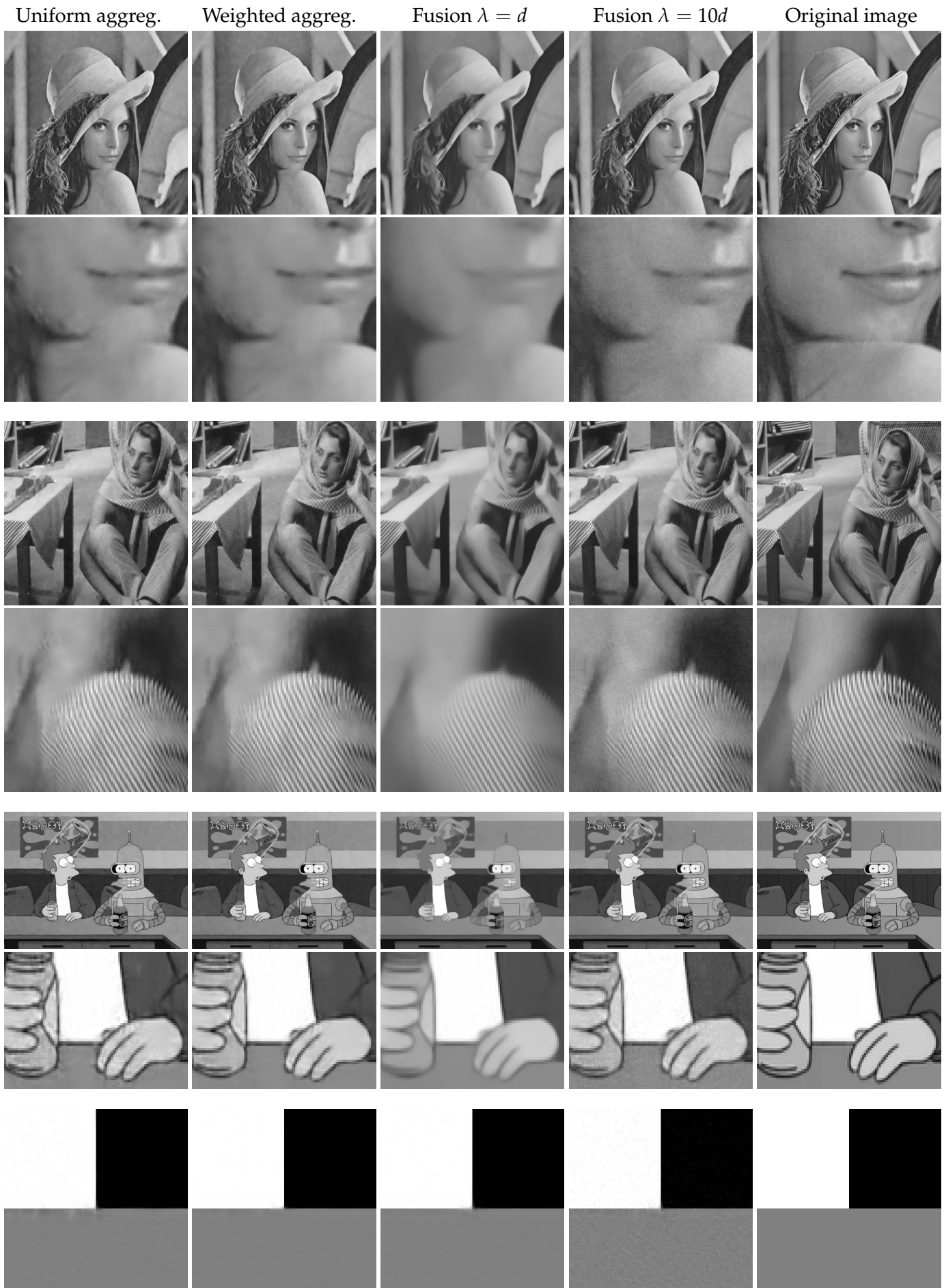
FIGURE 2.15: Comparison of the different aggregation procedures on the 4 test images, using HDMI for the inference of Gaussian models. Images are degraded by a noise of standard deviation \sigma = 30 .
