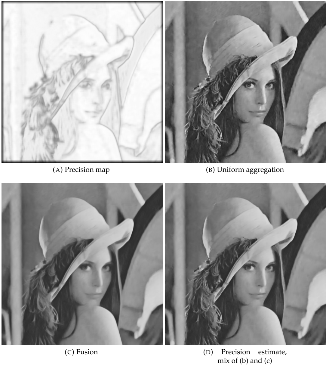
FIGURE 2.19: The inverse of the diagonal of the covariance matrix gives us the precision of the marginal of each pixel. This is a basic estimate of how confident the model is for each pixel. This enables to compute the precision estimate, which tries to keep the best of both worlds.
