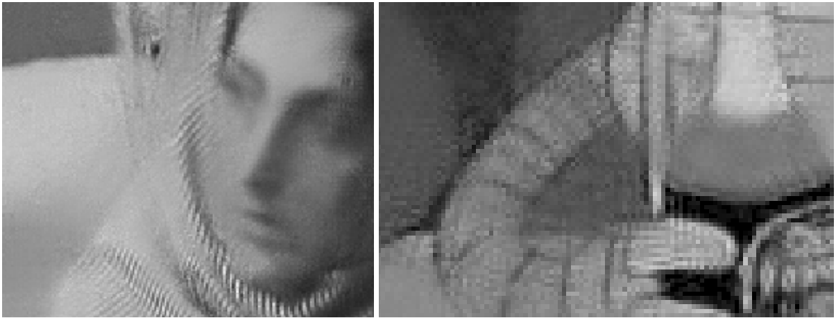
FIGURE 2.1: Issues on the reconstruction of Barbara and Cartoon with the NL-Means algorithm for \sigma = 50 . As we can see, the images contains strong artifacts, especially around the borders.
