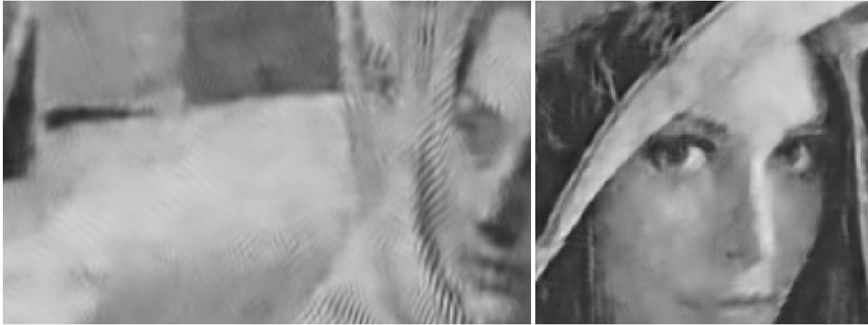
FIGURE 2.4: Issues on the reconstruction of Barbara and Cartoon with the HDMI algorithm for \sigma = 50 . We can see on Barbara that the stripes are well-denoised, but they are still (wrongly) visible on the floor and in the door. On Lena , there is no such defect, but a strong fluffy effect.
